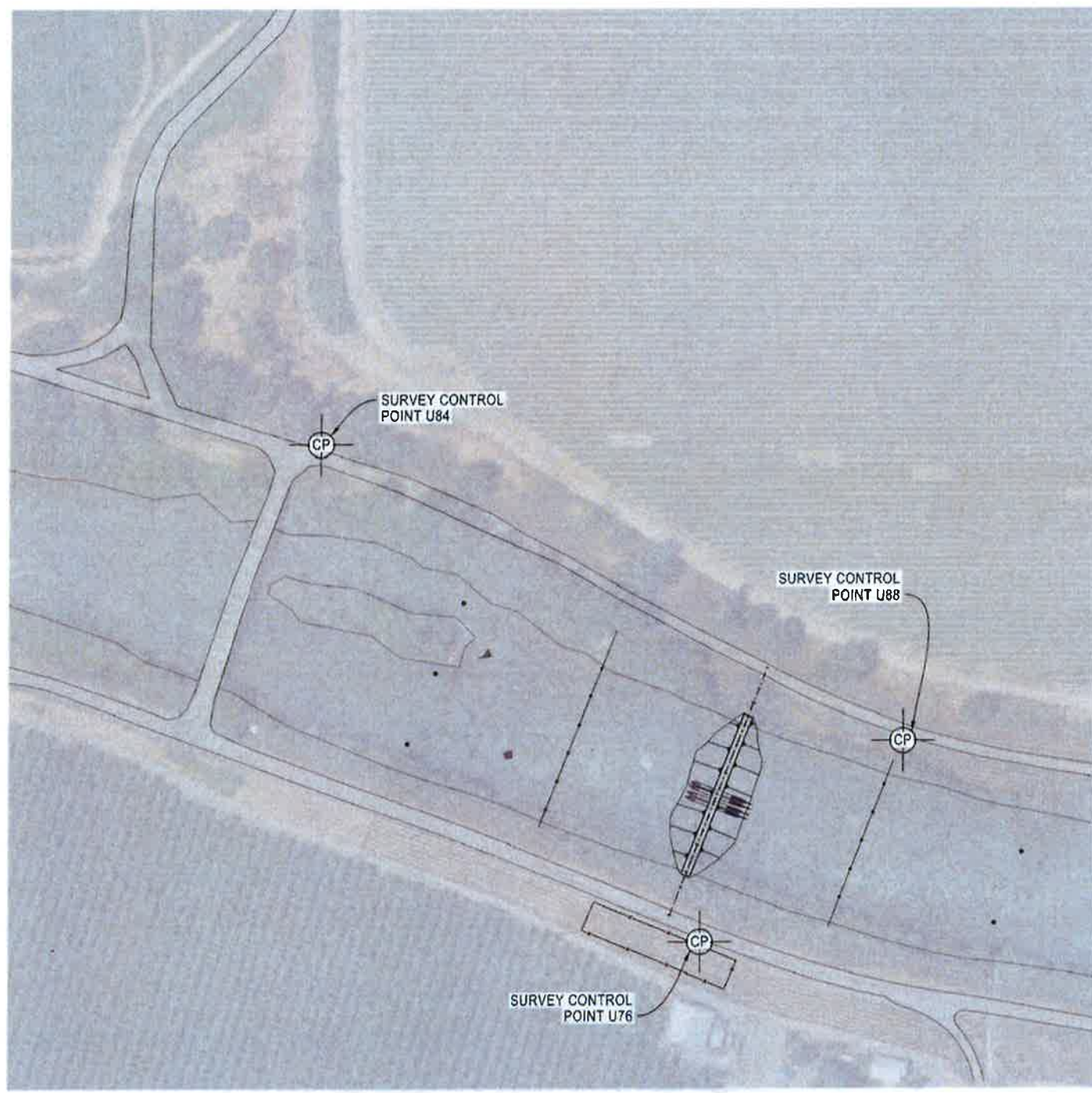
MINER SLOUGH - SURVEY CONTROL PLAN SCALE: 1" = 100'-0"
