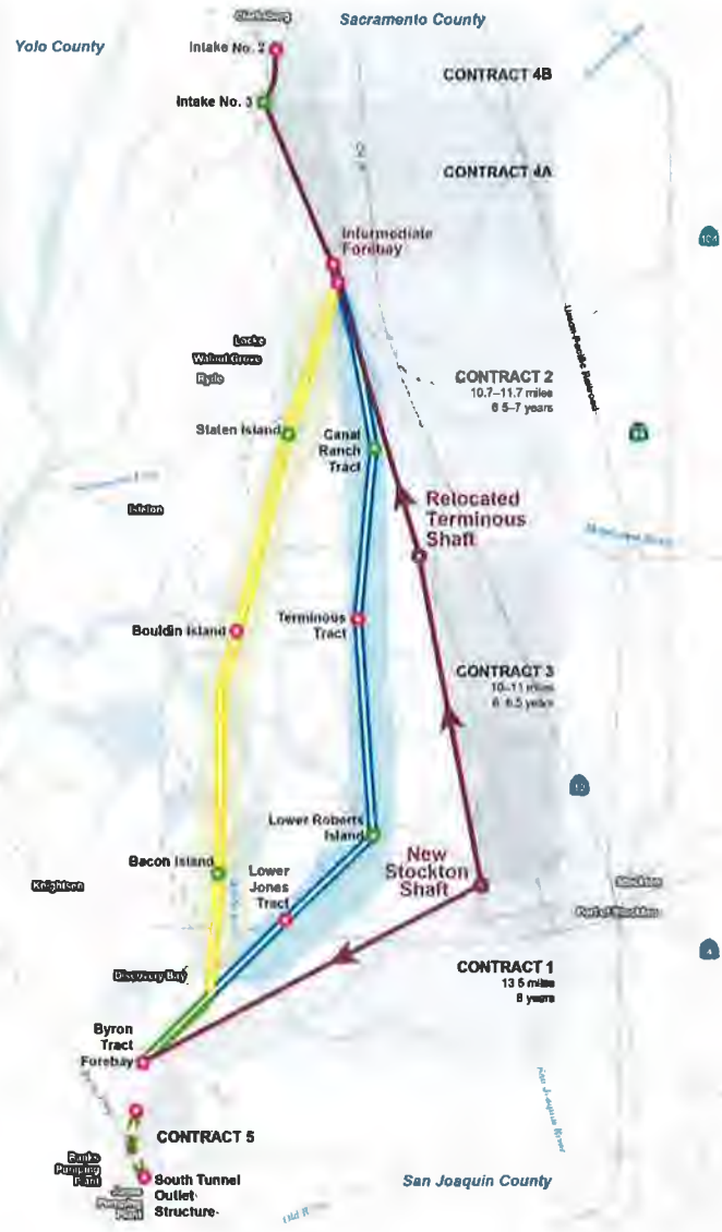
Figure 8. Recommended Tunnel DB Contract Packaging
